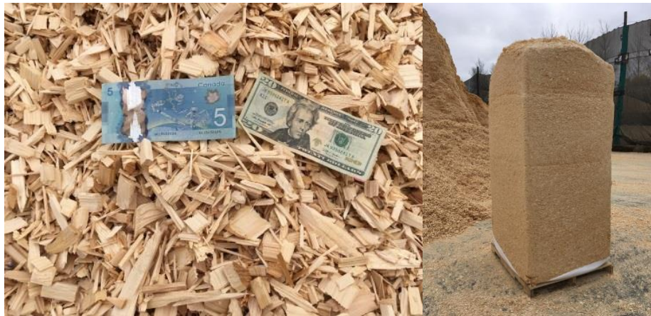
Example of raw fiber before densification and after. Solid as a brick.
